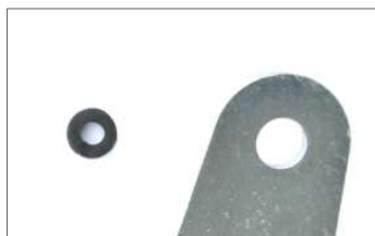
Fig. 2: If the rear wheel is equipped with a screw axle, remove the inserted adapter ring from the axle mount of the adapter.
