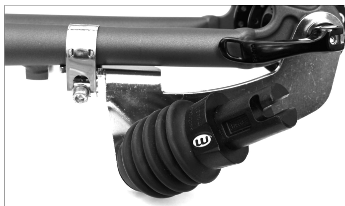
Fig. 4: Adapter with Weber coupling mounted on a wheel with quick-release axle (in the picture for a better overview without rear wheel).
