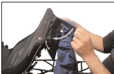
Schutzhuse an Tasche ankletten Connect raincover with the velcro on the bag
