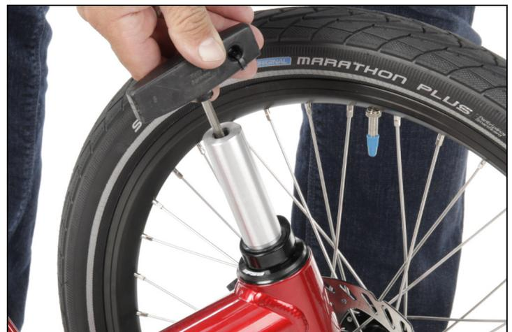
*Fixing the inserted knuckle adapter*
